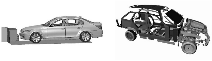
Fig. 2. Recent model of BMW employed for data mining (left). One FE input deck consisting of numerous parts (right)
